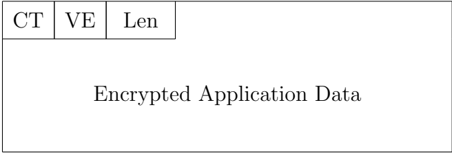
Figure 3.18: Logical structure of an Application Data Message
