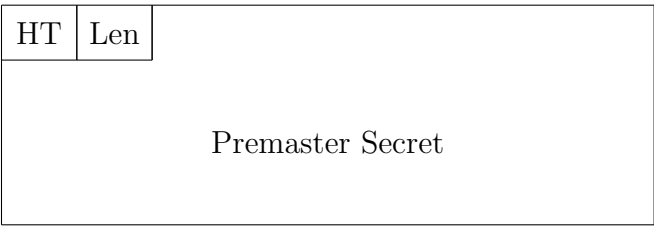
Figure 3.14: Logical Structure of a Client Key Exchange Message
