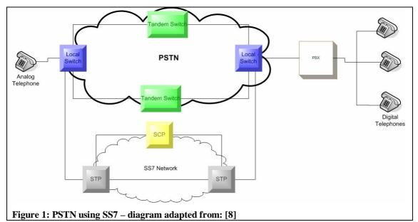
Figure 1 illustrates how the components of a PSTN are connected to provide a communication service. Taking these components into consideration VoIP should not only replicate but better the current structure of PSTNs so as to make it more scalable, attractive and efficient. Similar to what the telephone was to the telegram, VoIP is to the telephone. For VoIP to work there must be a seamless marriage between PSTNs and data networks (the Internet).
