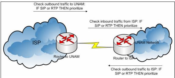
Figure 7: Traffic shaping between UNAM and ISP
