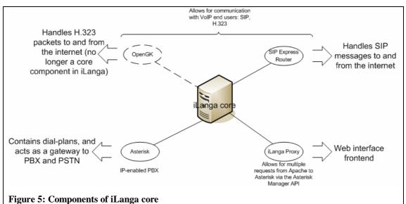
In Figure 5 it should be noted that OpenGK is no longer in use as iLanga prefers SIP agents over H.323 agents. The iLanga core is a suitable fully functional PBX to implement for VoIP deployment and that is why we will be using it for this project.
