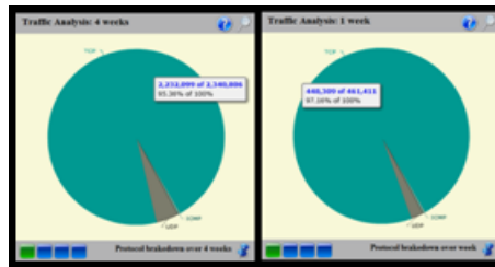
Figure 4.5: Protocol Breakdown, pie chart showing the proportion of TCP, UDP and ICMP packets captured over two intervals.
