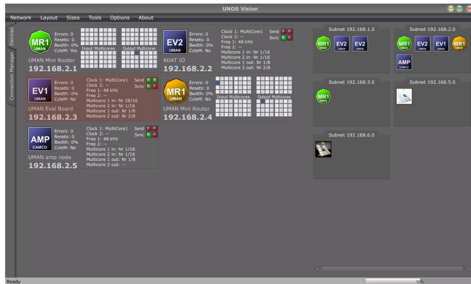
Figure 3: Small network configuration as it appears in UNOS Vision [20]
