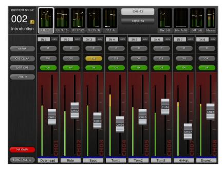
Figure 3.4: Yamaha Stage Mix iPad application for the LS9 digital mixing console. Image from www.yamaha.com .
