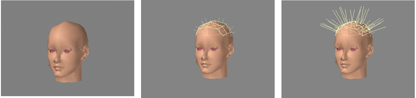
Figure 1: The modeling process to “grow” hair on the scalp using the HairDesign plug-in. A head model is designed or imported (left), the user selects the polygons on which they want hair to be placed (middle), and run the HairDesign plug-in. The plug-in produces control hairs (right).
