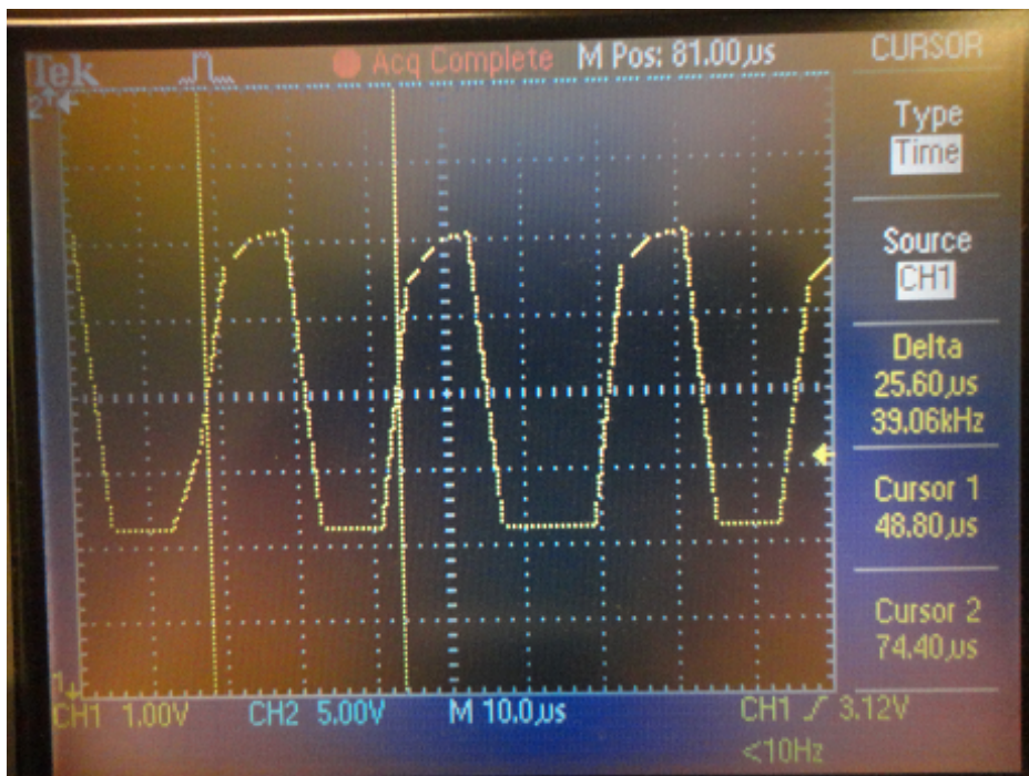
Figure 4.4: The carrier frequency shown on an oscilloscope.
