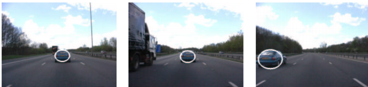
Figure 2.1: Results from the study by [26] where colour distributions and particle filtering were used to track a car.
