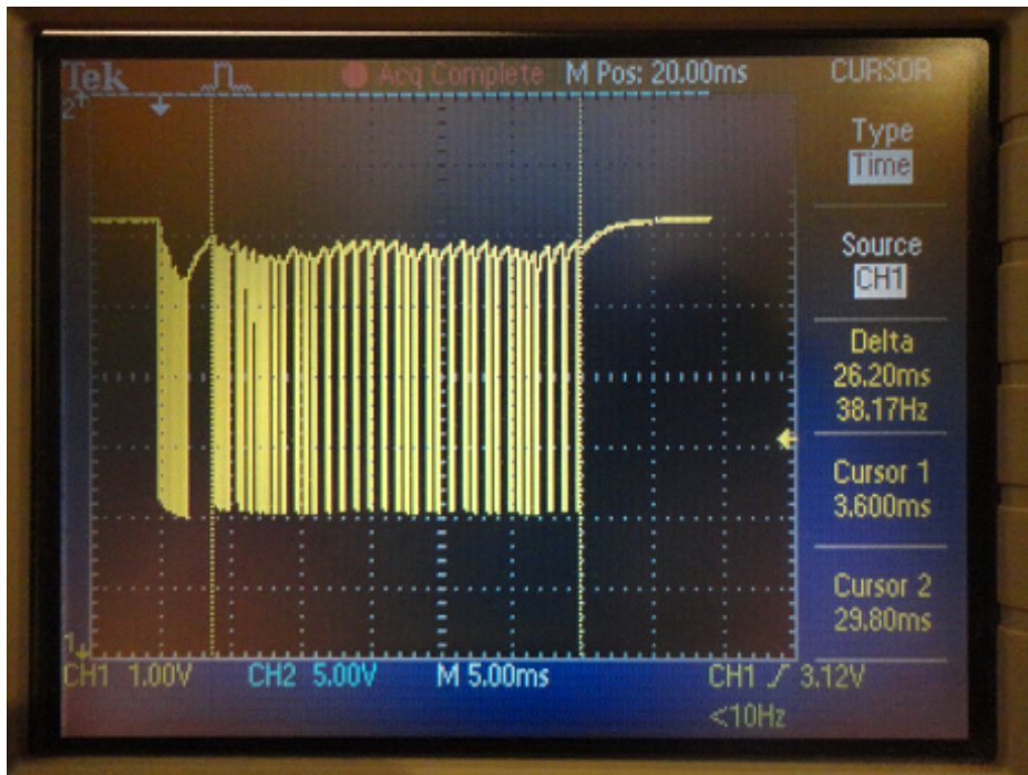
Figure 4.3: A full infrared packet shown on an oscilloscope.
