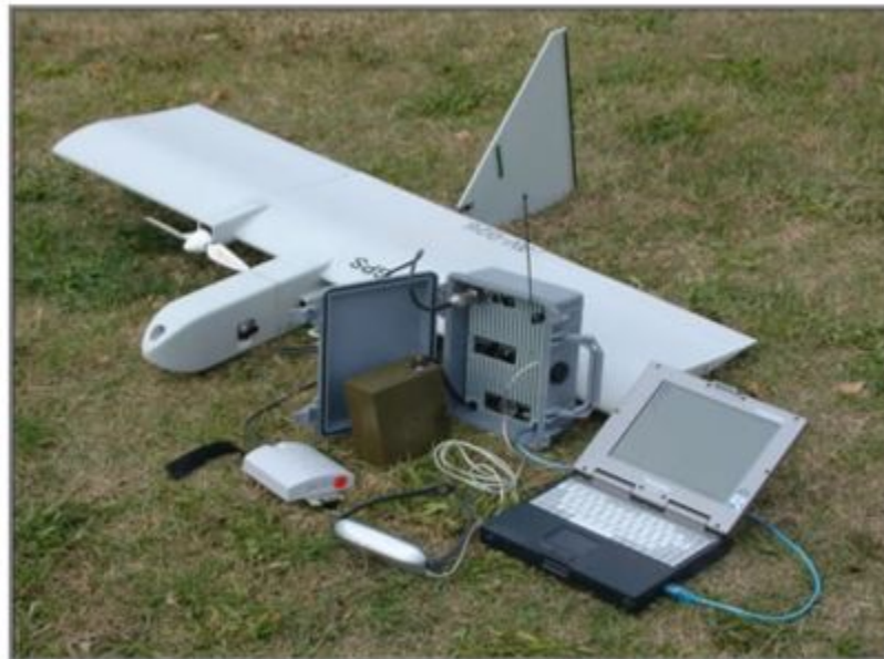
Figure 2.1: The Dragon Eye. A micro UAV (Arjomandi et al. , 2007)
